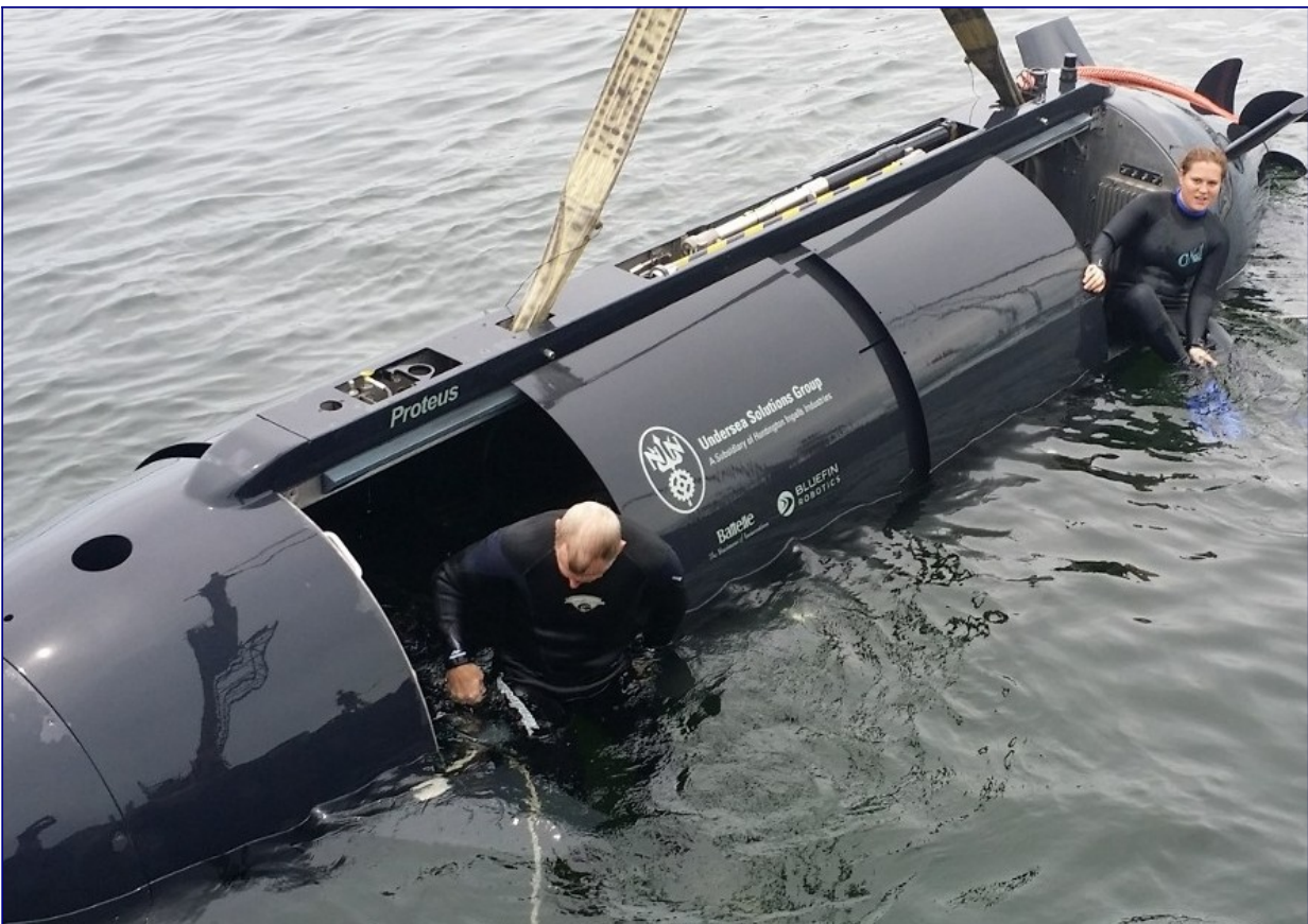
IMAGE: PROTEUS Dual-mode underwater vehicle (DMUV) taken out for a test in Florida's Saint Andrews Bay – USG Vice President Ross Lindman as the pilot
